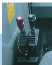
The crane operating levers are of finger control type and surely and steadily respond to the operator.
