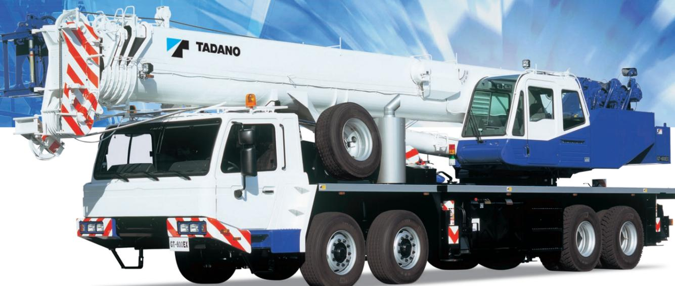
The adoption of a new hydraulic suspension system has enabled fast and comfortable road travel. The GT-600EX is a truck crane made in Japan, with a crane capacity of 60 metric tons, featuring a new design that reduces load and meets the Australian bridge formula.
