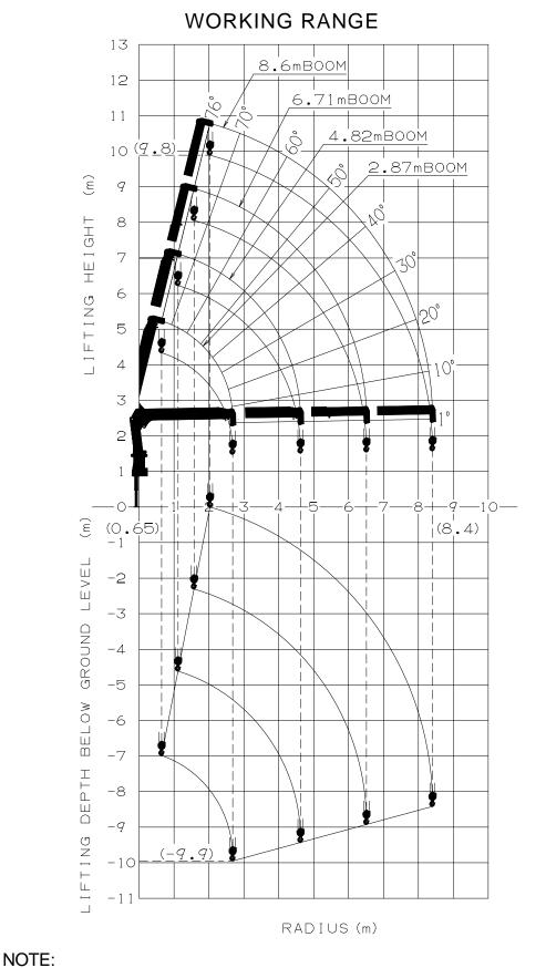
The above lifting heights and boom angles are based on a straight (unladen) boom, and allowance should be made for boom deflection obtained under laden conditions.
